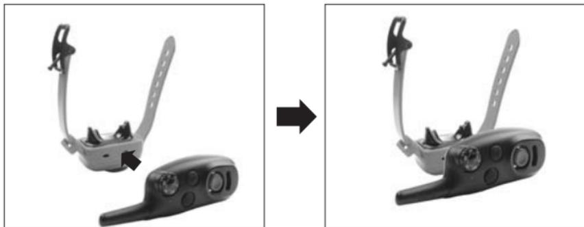
To activate the receiver/collar, place the red dot on the back of the handheld transmitter to the red dot on the receiver/collar. Hold the two red dots together for a moment until the LED light on the receiver/collar comes on.
